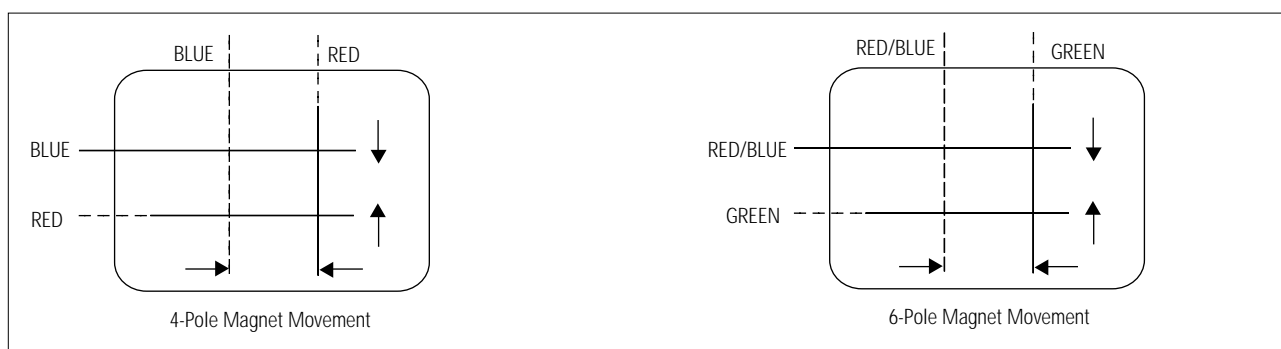
Fig. 4-5 Center Convergence Adjustment
